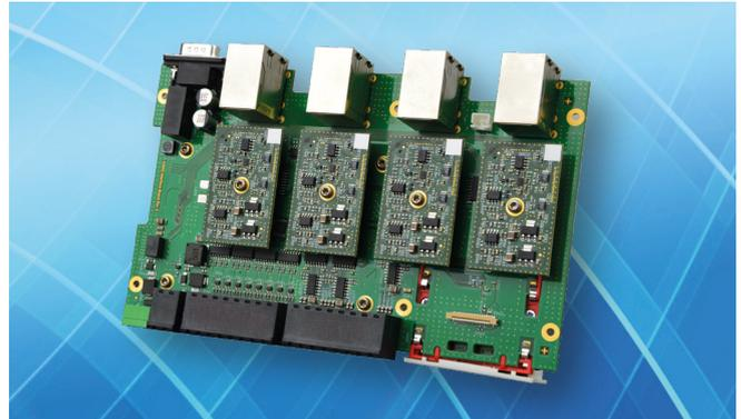
PCB of the unit with a view of the four interchangeable interface boards.
