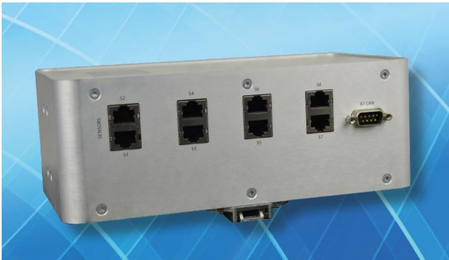
Top view with connections for network, fieldbuses and digital/ analogue inputs.
